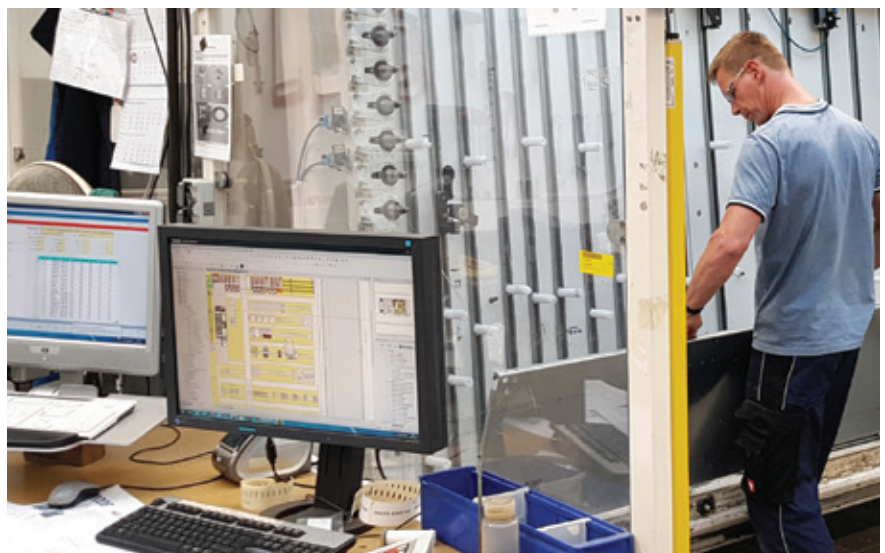
Cabinet layouts, including all the production data for labelling, wires and cabinet enclosures, are generated without any additional licence costs using the Cabinet Engineering Expert module and sent to the NC machines of renowned manufacturers.
