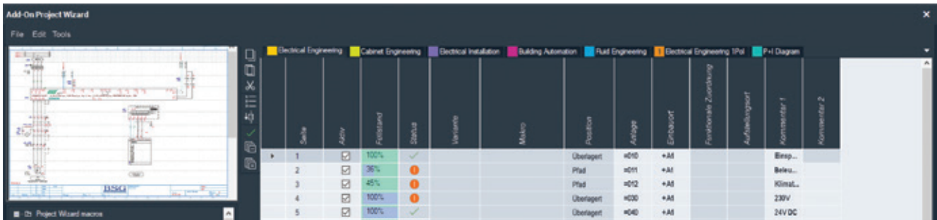
Circuit diagrams, cabinet layouts and documentation are generated automatically in WSCAD via the "Project Wizard" add-on. Time savings of up to 30 per cent are achieved in respect of the engineering for individual plants and up to 90 per cent for standard control systems.
