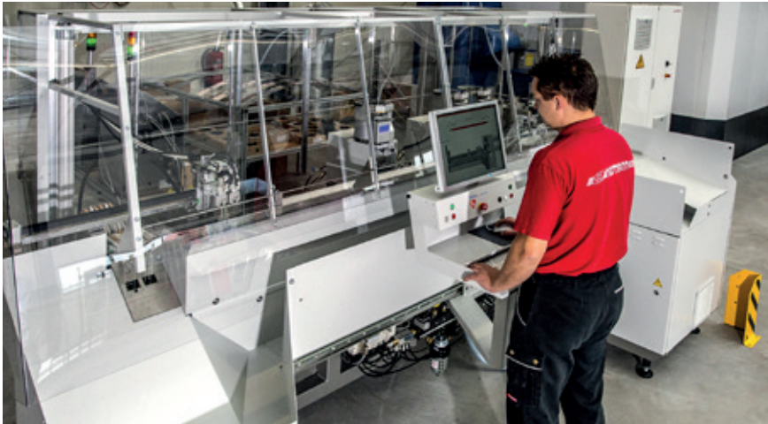
For the production of wires and wire sets, the NW-Niemann GmbH has invested in an NC machining center from Komax – the data for this comes directly from the cabinet layout created with the WSCAD software.
